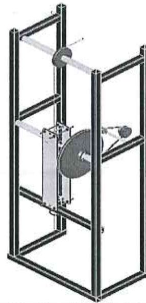
Fig. 2. Gym equipment with chain sprocket mechanism (bicep/ triceps machine)
